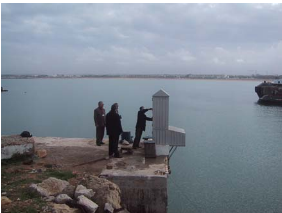
Figure 22, Mohammedia Port Radar Tide Gauge
