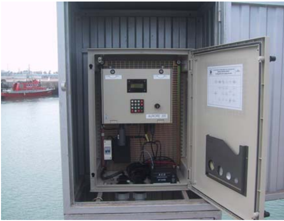
Figure 20, Mohammedia DPDPM Warsh/Martech Radar Tide Gauge. Data cartridge is the grey cylinder at the base of the Aurore 200 data logger.
